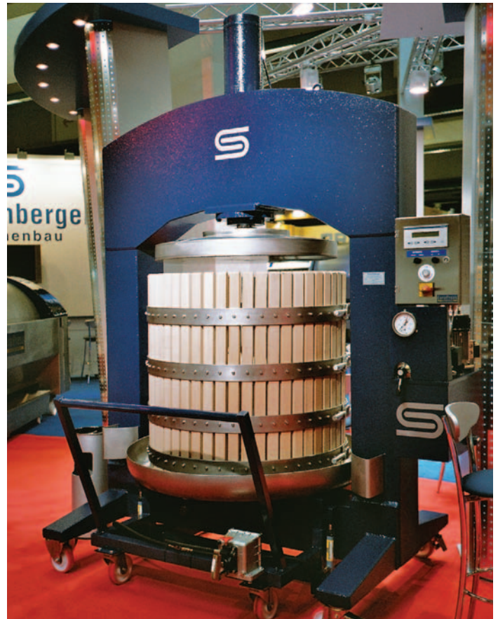
The Europress EVP structure is built from industry-standard enameled mild steel, but an all stainless steel press frame is available. A fully automatic digital control system is also available as an option.
